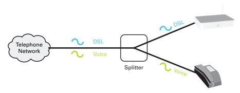
A filter between your telephone outlet and your phone. This filter removes the DSL signal and passes the Voice signal.
